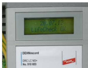
Interval testing with DRC LC M3+.
