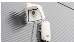
IP66 version suitable for outdoor use.
